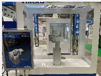
DD(Direct-Drive) Wafer atmospheric transport robot
