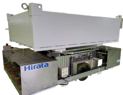
1 ton-type AGV (test unit) - Lift (100 mm), Rotating platform (±90°) - Capable of transporting up to a 1,400 kg load when a pallet is used
