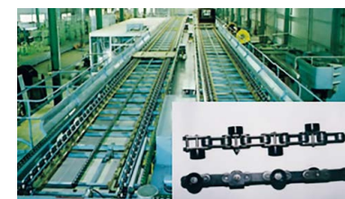
"MEP Chain" Conveyor A worker-focused free flow system where products stop moving in front of line workers so that they can be assembled, etc.
