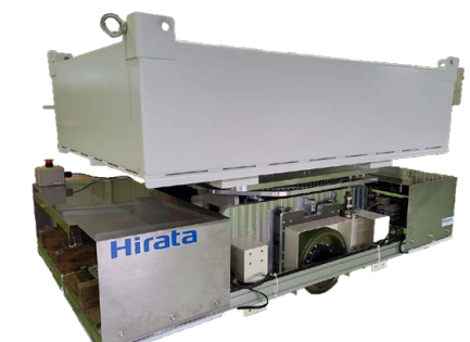
1 ton-type AGV (test unit) - Lift (100 mm), Rotating platform (±90°) - Capable of transporting up to a 1,400 kg load when a pallet is used
