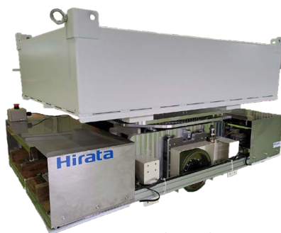
1 ton-type AGV (test unit) - Lift (100 mm), Rotating platform ( \pm 90^\circ ) - Capable of transporting up to a 1,400 kg load when a pallet is used
