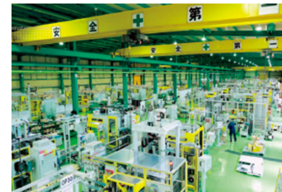
EDU(Electric Drive Unit) 組立設備
