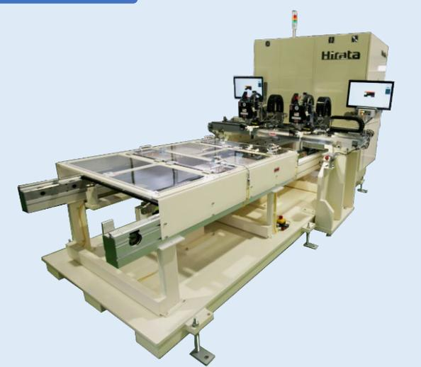
**Wire bonding machine with dual head**
