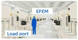
Multiple EFEM/load ports are used on a single line because multiple EFEM/load ports are installed at each processing unit.
