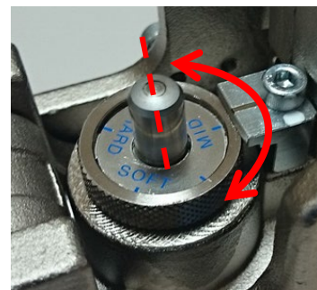
Fig. 2.9 Dial for Adjusting Shock Absorber Reaction (EST50 and 80)
