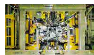
Cold tester Comprehensive engine testing without the need for combustion
