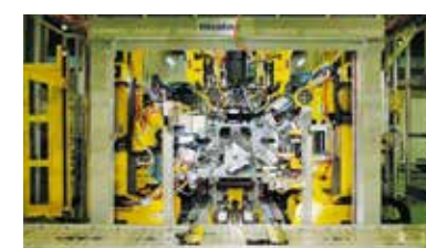
Cold tester Test under the condition of non-combustion
