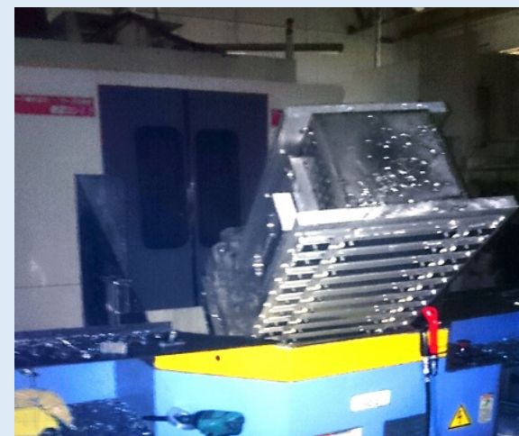
Fallen jigs over processing machine
